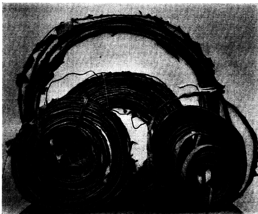
Fig. 4. Coils used by Henry in his experiments on electromagnetic induction.
