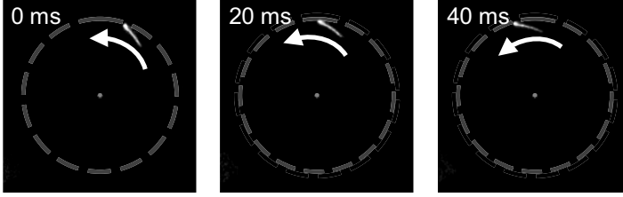
(b) Double-wave rotating flame f = 3.5 \text{ Hz} @ \dot{V}_{\text{in}} = 10.63 \text{ SLPM} , \phi = 1.25
