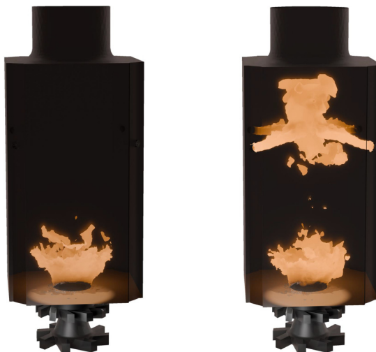
FIG. 2. Instantaneous temperature isosurfaces ( T = 1350 K) for cases without (left) and with (right) dilution jets.
