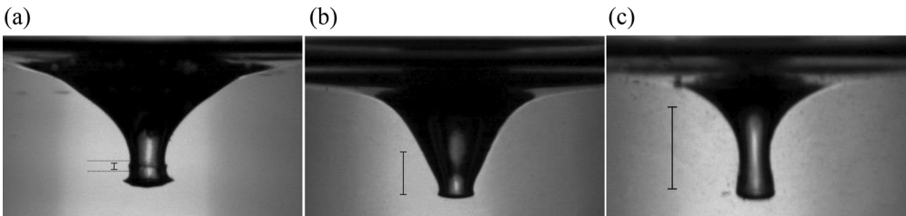
FIG. 5. Cavity shapes at \tau = 1 ms (a) water, (b) GW 80, and (c) GW 90. The calculated wavelengths \lambda are indicated by the vertical lines. The dotted horizontal lines in (a) shows the measured wavelength.
