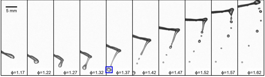
FIG. 12. Downward Euler droplet ejection, observed upon impact of a drop D2 at 15 mm from the tip of leaf L24 (period 102 ms). The phase \phi at which snapshots were taken is reported at the bottom. The scale bar is 5 mm. The first droplet in this burst is framed in blue at the time it is ejected. The corresponding movie is available in the Supplemental Material [46].
