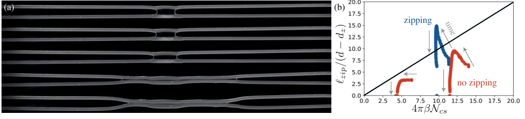
FIG. 9. Swelling-induced zipping. (a) Chronophotography of the absorption of a silicone oil drop ( \eta = 2 mPa s) between two VPS 32 fibers of radius r = 250 \mu\text{m} (one picture every 200 ms). (b) Measured evolution of the deformation \ell/(d - d^*) as a function of the fiber tension through the capillary stretching number \mathcal{N}_{cs} . Here the tension is measured with a force sensor, and the other quantities are measured on photographs. Line given by Eq. (4).
