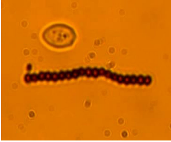
VIDEO 3. The video illustrates the transport of a colloidal ribbon close to a yeast cell via application of a precessing magnetic field, with frequency f = 50 Hz and amplitudes H_x = 0.3 Oe, H_y = 37.4 Oe, H_z = 3.5 Oe.
