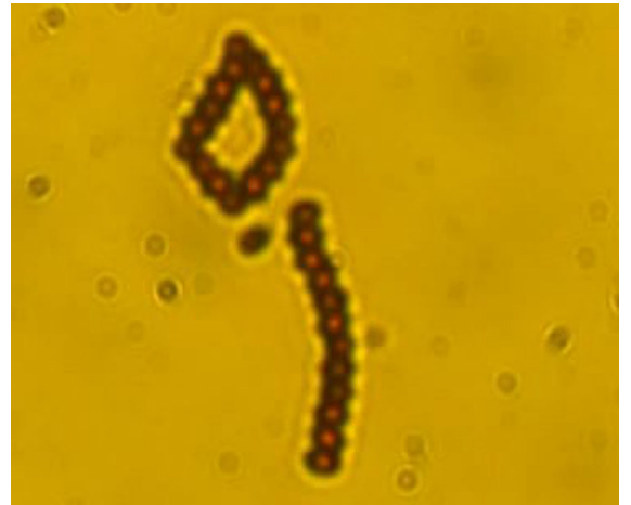
VIDEO 2. Dynamics of a ring and a close located ribbon when subjected to an external magnetic field applied along the x direction and with amplitude H = 0.7 Oe. The ring shrinks along the applied field, and the ribbon reorient along the field direction.
