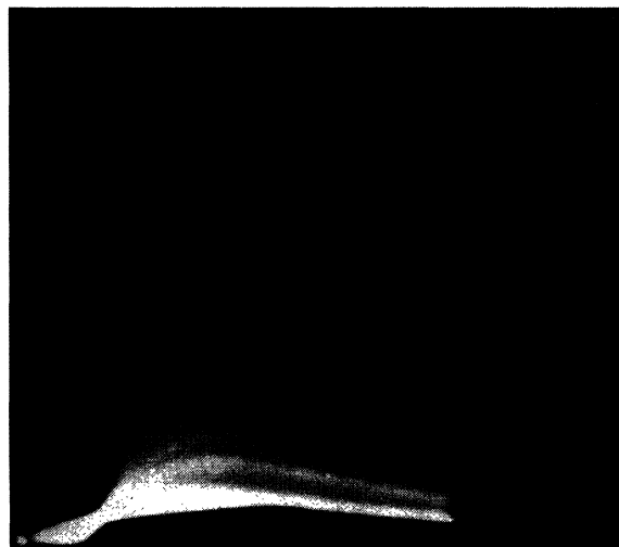
FIG. 1. Oscillogram of the Po-Be calibration spectrum, showing also photoelectron lines due to Po and a trace of Ra impurity.
