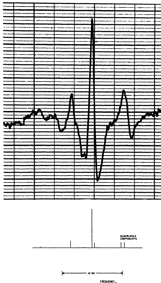
FIG. 1. Above: the experimental curve showing the partially resolved spectrum of COS 35 . Below: the theoretical pattern calculated for a spin of 3/2 for S 35 .
