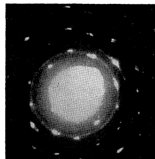
FIG. 3. A single diagram of the \text{Fe}_3\text{O}_4 specimen at 300°C. There is no splitting at the diffraction spots here.
